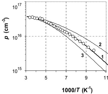
Fig.1 The hole concentration, by the Hall effect, for the compensated sample 44c (open circles). The thick solid curve 1 is computed with the best-fit values of  $N_a$  and  $N_d$  ( $N_d/N_a = 0.41$ ). The thin solid curves are computed with a different compensation degree:  $N_d/N_a = 0.2$  (curve 2) and  $N_d/N_a = 0.6$  (curve 3).
