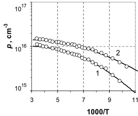
Fig.2 The hole concentration deduced from the Hall effect in compensated sample 45c (curve 1) and non-compensated one 72nc (curve 2). The solid curves are computed with the best-fit values of  $N_a$  and  $N_d$ ; for 45c they are shown in Table 1, for 72nc they are  $N_a = 1.6 \times 10^{16} \text{ cm}^{-3}$ ,  $N_d = 7.8 \times 10^{14} \text{ cm}^{-3}$ .
