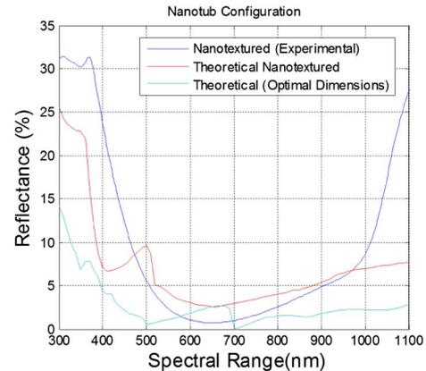
Fig. 8. Experimental and theoretical data with AR coating. The reflectance from the 900–1100 nm region is due to reflection from the rear of the wafer, which is not included in the simulated structure.
