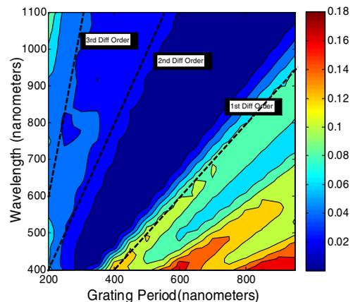
Fig. 5. Reflectance of nanotub structure without AR coating with aspect Ratio = 0.69. The first through third diffraction orders are also plotted indicating optimal light in-coupling between orders 1 and 2.
