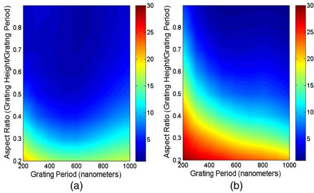
Fig. 6. Total SWR for nanotub and pyramid structures at aspect ratios for 200–950 nm periods with AR coating. Significantly lower reflectance could be observed for nanotubs with lower periods and high aspect ratios.
