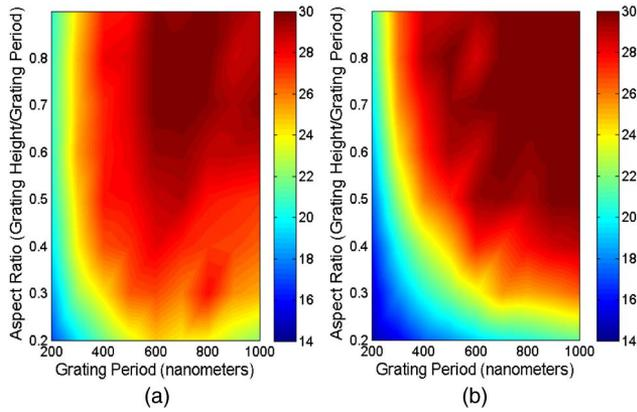
Fig. 3. Short-circuit current density  $J_{sc}$  ( $\text{mA}/\text{cm}^2$ ) of (a) nanotubs and (b) pyramids as a function of grating period and aspect ratio with nitride AR coating at a substrate thickness of  $3\ \mu\text{m}$ . Nanotubs still have higher current at lower aspect ratios spanning 0.2–0.4, but lower maximum current performance.
