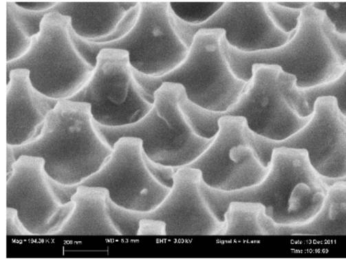
Fig. 7. SEM image of sample nanotubs 200 nm height and 513 nm in period.
