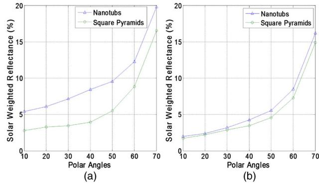
Fig. 4. SWR results for TE and TM averaged polar angles of incident light upon (a) non-AR coated and (b) AR coated cells.
