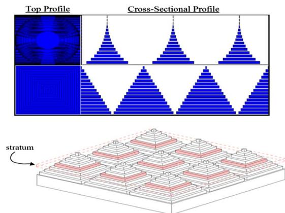
Fig. 1. Construction of diffraction grating, consisting of a substrate layered on top with a specified number of stratum. Blue represents the etched silicon and white represents air.
