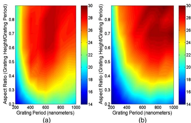
Fig. 2. Short circuit current density  $J_{sc}$  (mA/cm<sup>2</sup>) of (a) nanotubs and (b) pyramids as a function of grating period and aspect ratio without nitride AR coating at a substrate thickness of 3 μm. Nanotubs have higher current at lower aspect ratios spanning 0.2–0.4.
