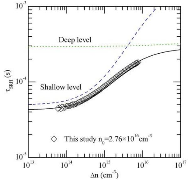
Fig. 2. Measured injection level dependence of the SRH lifetime for a compensated n-type silicon sample ( $n_0 = 2.76 \times 10^{16} \text{ cm}^{-3}$ ). The lines are fits using the SRH equation. The dotted line represents the effect of the deep level, while the dashed line represents the effect of the shallow level. The solid line represents their combined impact.
