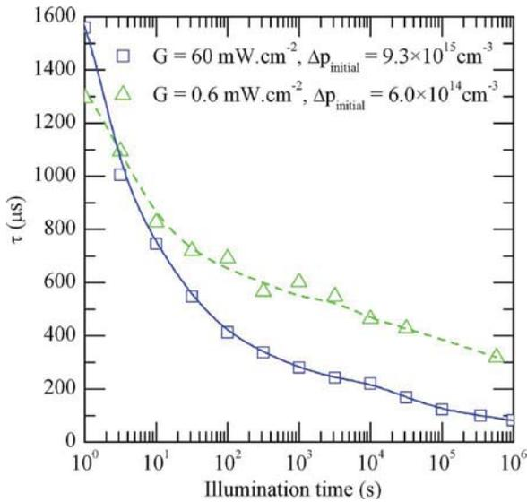
Fig. 6. Evolution of the effective lifetime during BO generation in compensated n-type silicon for two different carrier generation rates ( $G = 60 \text{ mW.cm}^{-1}$ ,  $T = 60^\circ\text{C}$  and  $G = 0.6 \text{ mW.cm}^{-1}$ ,  $T = 30^\circ\text{C}$ ). The lines are guides to the eye.
