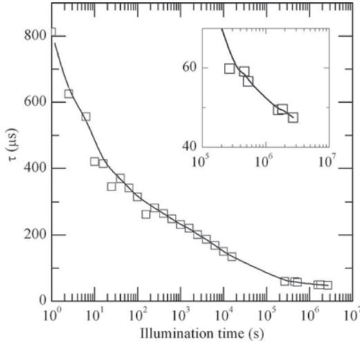
Fig. 1. Evolution of the effective lifetime during BO generation in compensated n-type silicon ( $n_0 = 1.9 \times 10^{15} \text{ cm}^{-3}$ ,  $G = 60 \text{ mW}\cdot\text{cm}^{-2}$ ,  $T = 60^\circ\text{C}$ ). The line is a guide to the eye.
