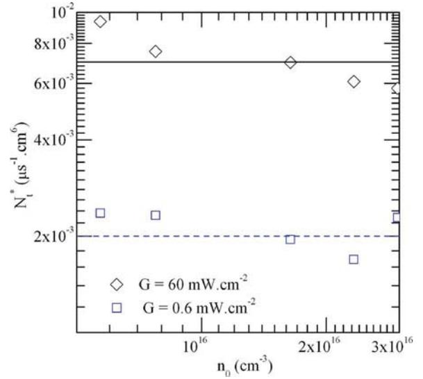
Fig. 7. Defect density in compensated n-type silicon for two different generation rates ( $G = 60 \text{ mW.cm}^{-1}$ ,  $T = 60^\circ\text{C}$  and  $G = 0.6 \text{ mW.cm}^{-1}$ ,  $T = 30^\circ\text{C}$ ). The lines are guides to the eye.
