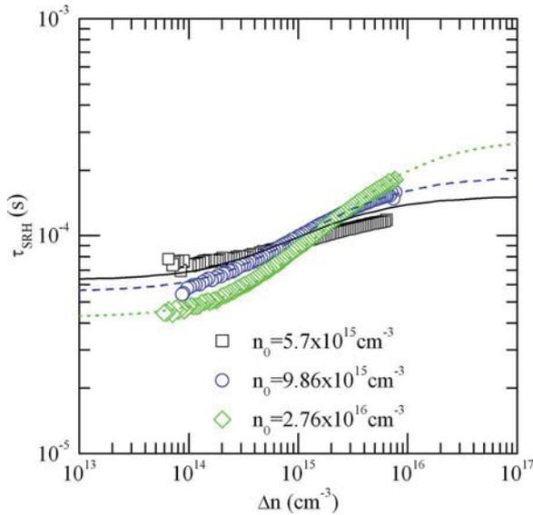
Fig. 4. Measured injection level dependence of the SRH lifetime for three different samples ( $n_0 = 5.7 \times 10^{15}$ ,  $9.86 \times 10^{15}$ , and  $2.76 \times 10^{16} \text{ cm}^{-3}$ ). The lines are fits using the SRH equation with a deep and shallow level.
