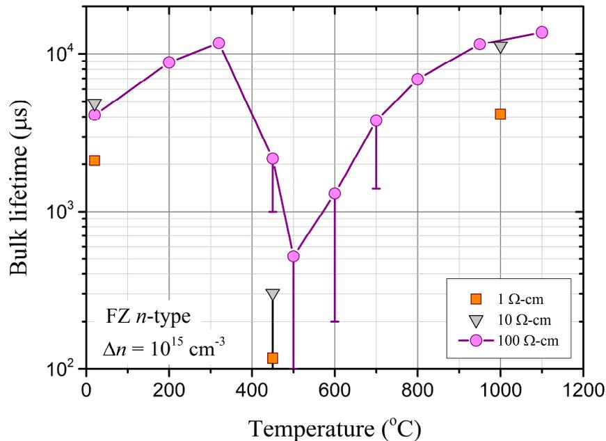
Figure 1: Bulk lifetime (at  $\Delta n = 10^{15} \text{ cm}^{-3}$ ) versus annealing temperature for three different FZ silicon wafers, 1  $\Omega$ -cm, 10  $\Omega$ -cm and 100  $\Omega$ -cm. Annealing was performed in oxygen for 30 mins. For each annealing temperature, new samples were used. The bulk lifetime was measured using HF passivation [8].
