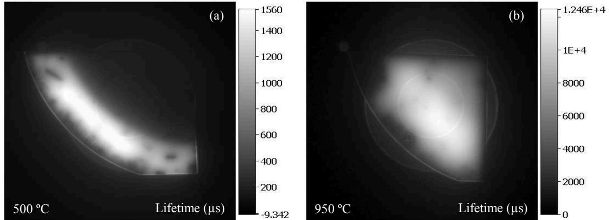
Figure 2: Calibrated photoluminescence images of  $\text{Al}_2\text{O}_3$  passivated 100  $\Omega$ -cm silicon samples which were previously annealed at (a) 500  $^\circ\text{C}$  and (b) 950  $^\circ\text{C}$  in oxygen for 30 mins. Note the different lifetime scales.
