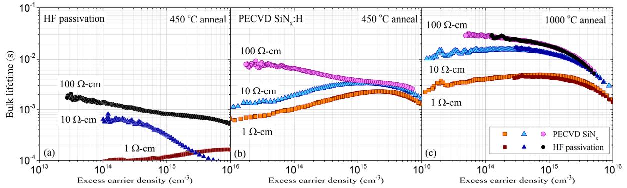
Figure 3: plots the bulk lifetime of FZ  $n$ -type samples after annealing at 450 °C in  $O_2$  for 30 mins (a) followed by a HF passivation measurement, (b) after a subsequent PECVD  $SiN_x:H$  deposition and (c) after stripping the  $SiN_x:H$  film and subsequently annealing the samples at 1000 °C in  $O_2$  for 30 mins. Following the high temperature anneal, the samples were measured with HF passivation and then coated with PECVD  $SiN_x:H$  once again.
