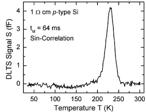
FIG. 1. DLTS spectrum of the Mn-contaminated 1  $\Omega$  cm sample for a sine correlation function.
