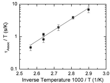
FIG. 8. Arrhenius plot of the association time constant for the intentionally Mn-contaminated 20  $\Omega$  cm sample. From the fit, the prefactor  $A$  (and hence the diffusion coefficient  $D_0$ ) and the migration enthalpy  $H_M$  were determined.
