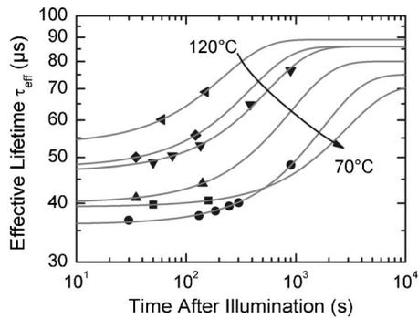
FIG. 7. Effective lifetimes measured by means of MW-PCD after the Mn-contaminated 20  $\Omega$  cm sample has been illuminated with white light ( $I_{\text{bias}} = 0.3$  W/cm $^2$ ) for at least 5 min. For every temperature, an exponential fit resulted in the (temperature-dependent) association time constant  $\tau_{\text{assoc}}$ . Please note that  $\tau_{\text{assoc}}$  is independent of the percentage of broken MnB pairs directly after illumination.
