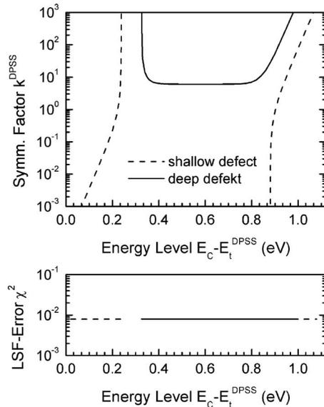
FIG. 4. DPSS analysis of the IDLS curve of the Mn-implanted 20  $\Omega$  cm sample. The errors  $\chi^2$  and ratios of the capture cross sections  $k$  of the IDLS fit for the shallow and the deep defect center are plotted for a fixed but gradually varied energy level  $E_C - E_t$ . Each parameter set for the shallow and the deep level from the diagram give the same good fit, as can be seen from the  $\chi^2$  error.
