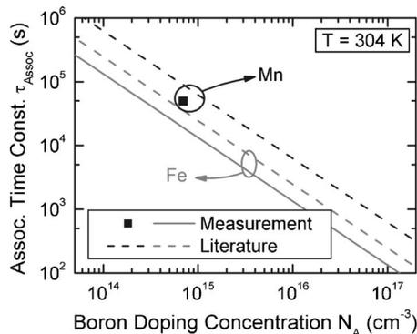
FIG. 9. Association time constant vs doping concentration determined for a temperature of  $T=304$  K for iron (Ref. 31) and manganese (this work). The comparison shows the calculated values based on the diffusivity and activation energy taken from literature and the measured data.
