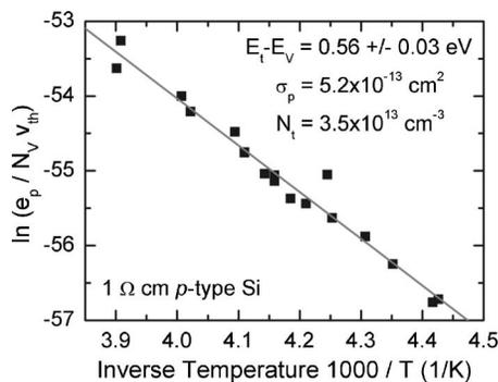
FIG. 2. Arrhenius plot of the DLTS data for the 1  $\Omega$  cm sample. In the inset, the extracted defect parameters are shown.
