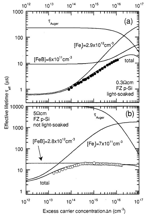
FIG. 3. Examples of the fitting procedure for the effective lifetimes for: (a) the 0.3  $\Omega$  cm sample with light soaking, and (b) the 5  $\Omega$  cm sample without light soaking. The constituent curves for Fe<sub>i</sub>, FeB pairs, and Auger recombination are shown for each plot, and the concentrations of the recombination centers used for the fits are given in Table II. In both cases, the implanted dose was  $1 \times 10^{11} \text{ cm}^{-2}$ .
