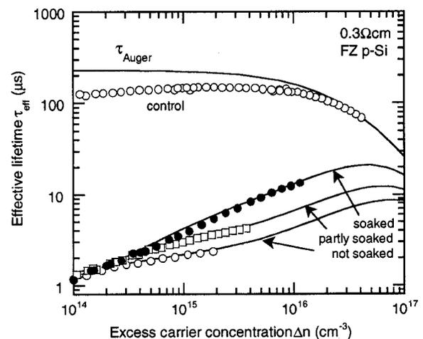
FIG. 4. Lifetime measurements (symbols) and SRH fits (solid lines) for the 0.3 Ω cm sample implanted with an iron dose of 1×10<sup>11</sup> cm<sup>-2</sup>. Three curves corresponding to different light soaking levels are shown. The concentrations of Fe<sub>i</sub> and FeB pairs used to generate the fits are given in Table II, and the recombination parameters in Table I.
