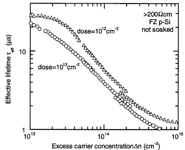
FIG. 7. Lifetime measurements for high resistivity ( $>200$   $\Omega$  cm) samples implanted with iron doses of  $1 \times 10^{12}$   $\text{cm}^{-2}$  and  $1 \times 10^{13}$   $\text{cm}^{-2}$ . The small difference in recombination lifetimes reflects precipitation of iron during annealing.
