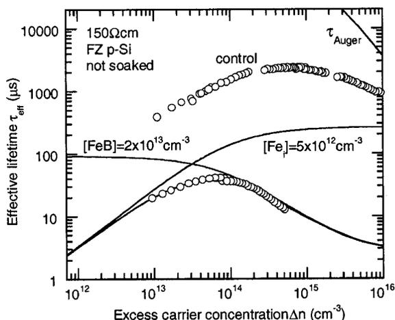
FIG. 6. Lifetime measurements (symbols) and SRH fit (solid lines) for the 150  $\Omega$  cm sample implanted with an iron dose of  $1 \times 10^{12}$   $\text{cm}^{-2}$ . The curve shown is for no light soaking. The concentrations of  $\text{Fe}_i$  and  $\text{FeB}$  pairs used to generate the fit are given in Table II, and the recombination parameters in Table I.
