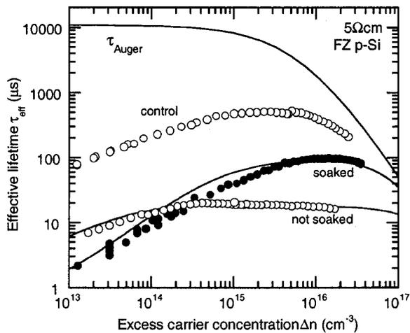
FIG. 5. Lifetime measurements (symbols) and SRH fits (solid lines) for the 5  $\Omega$  cm sample implanted with an iron dose of  $1 \times 10^{11}$   $\text{cm}^{-2}$ . Two curves corresponding to different light soaking levels are shown. The concentrations of  $\text{Fe}_i$  and  $\text{FeB}$  pairs used to generate the fits are given in Table II, and the recombination parameters in Table I.
