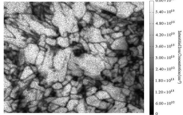
**Fig 3.** Interstitial Fe concentrations in an as-cut multicrystalline silicon wafer based on PL images. Sample width is 7 cm.
