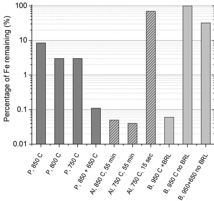
**Fig 6.** Fe gettering effectiveness for phosphorus (P), aluminium (Al) and boron (B) diffused regions for different diffusion conditions as explained in the text.
