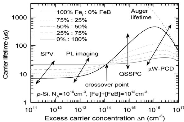
**Fig 2.** Modelled effective lifetimes for  $Fe_i$  and  $FeB$  pairs, and combinations of the two, as a function of excess carrier density.
