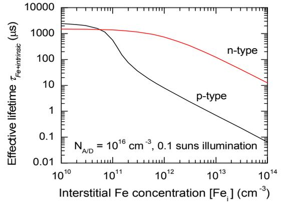
**Fig 1.** Effective lifetimes in n- and p-type Si as a function of the interstitial Fe concentration [Fe<sub>i</sub>].
