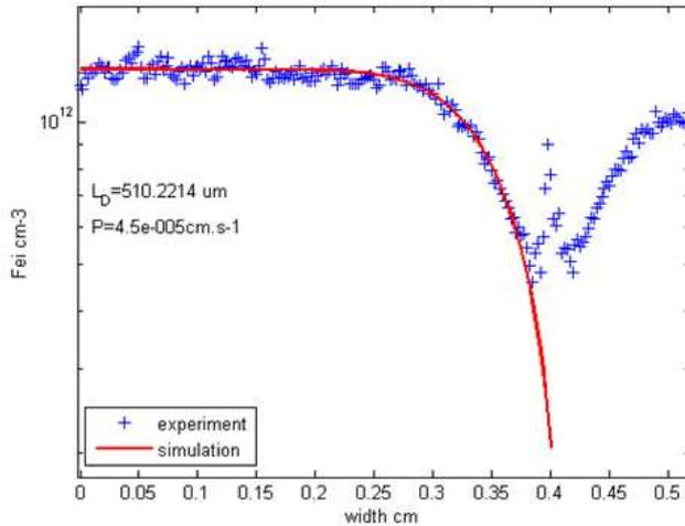
**Fig 4.** Linescan of the interstitial Fe concentration near a grain boundary in a multicrystalline silicon wafer which was annealed at low temperature. The red line shows a simple diffusion model fitted to the data, yielding a diffusion length of Fe during the precipitation process of 510 microns, and a precipitation velocity of  $4.5 \times 10^{-5}$  cm/s.
