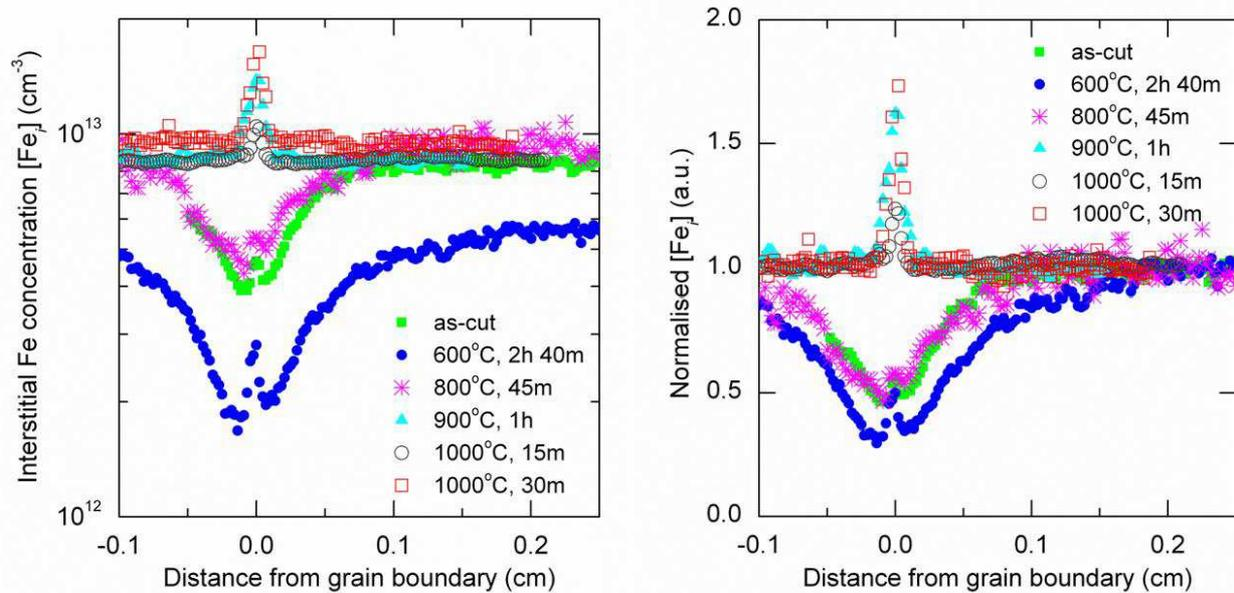
**Fig 5.** Linescans of the interstitial Fe concentration near a grain boundary in a mc-Si wafer after various annealing steps. The left hand plot shows the absolute interstitial Fe concentration, while the right hand plot is normalised far from the grain boundary, in order to allow changes in the relative width and depth denuded zone near the grain boundary to be more easily seen.
