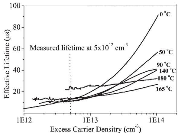
Figure 3. Lifetime curves of Fe-contaminated sample measured over a range of temperature for 100  $\Omega$  cm wafer
