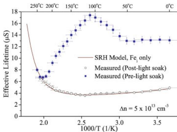
Figure 6. Arrhenius plot of effective lifetime SRH model and measured data for 1 Ω cm wafer
