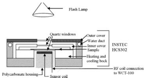
Figure 1. Experimental setup of PCD-based TIDLS system
