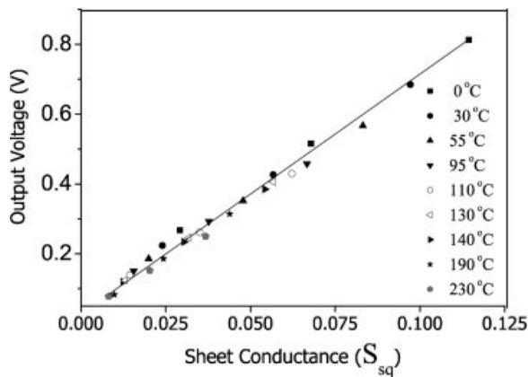
Figure 2. Calibration of the system for the sample temperature range, 0–230°C, under dark conditions
