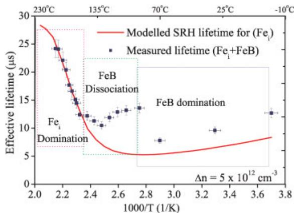
Figure 4. Arrhenius plot of lifetime SRH model and measured data for 100 Ω cm wafer
