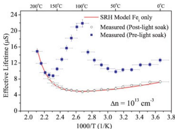
Figure 5. Arrhenius plot of lifetime SRH model and measured data for 13 Ω cm wafer
