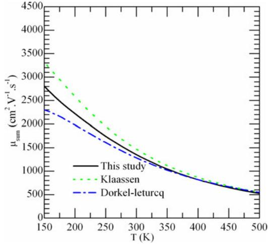
Fig. 8. Comparison of the empirical mobility sum from this study with the existing mobility models from Klaassen and Dorkel-Leturcq as a function of temperature at doping density of  $1 \times 10^{16} \text{ cm}^{-3}$  and injection level of  $1 \times 10^{16} \text{ cm}^{-3}$ .
