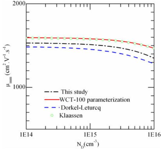
Fig. 7. Comparison of the empirical mobility sum from this study with the existing mobility models from WCT-100 parameterization, Klaassen and Dorkel-Leturcq as a function of doping density at 300 K and injection level of  $1 \times 10^{16} \text{ cm}^{-3}$ .
