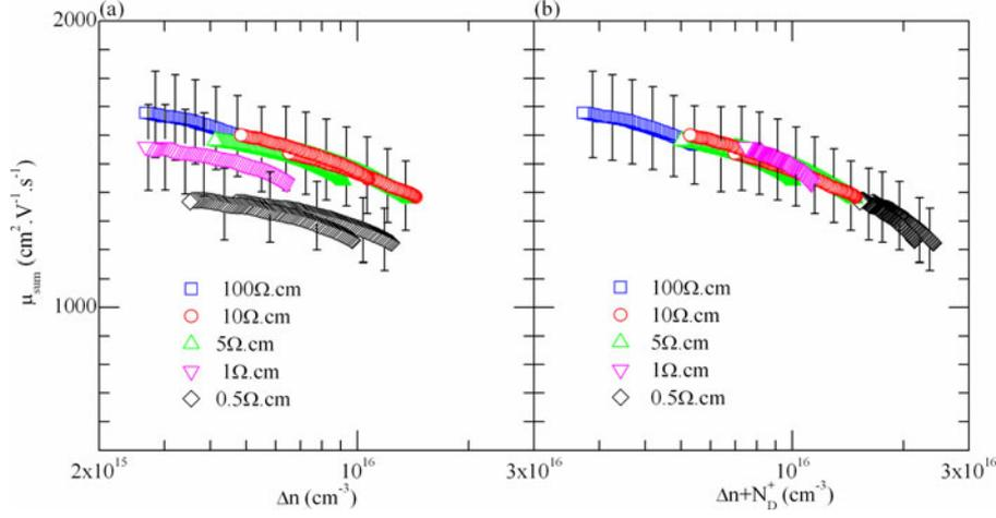
Fig. 1. (a) Measured mobility sum as a function of excess carrier density at 30 °C for five samples of different doping. (b) Measured mobility sum as a function of the sum of excess carrier density and the ionized doping density at 30 °C.
