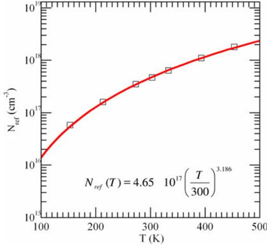
Fig. 5. Temperature dependence of the fitting parameter  $N_{\text{ref}}$ . This parameter is extracted from the experimental data and subsequently fitted using (5).
