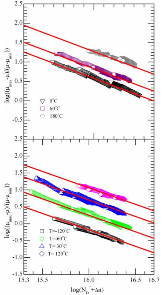
Fig. 3. Fitting of measured mobility sum using (3) at  $-120^\circ\text{C}$ ,  $-60^\circ\text{C}$ ,  $0^\circ\text{C}$ ,  $30^\circ\text{C}$ ,  $60^\circ\text{C}$ ,  $120^\circ\text{C}$ , and  $180^\circ\text{C}$ . The symbols are calculated based on the left hand side of (3), the solid lines are the fitting using the right hand side of (3) by adjusting  $N_{\text{ref}}$  and  $\alpha$ .
