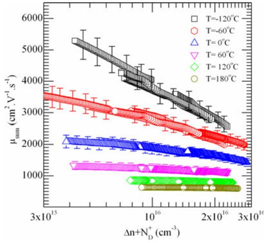
Fig. 2. Measured mobility sum as a function of the sum of excess carrier density and the ionized doping density at -120 °C, -60 °C, 0 °C, 60 °C, 120 °C, and 180 °C.
