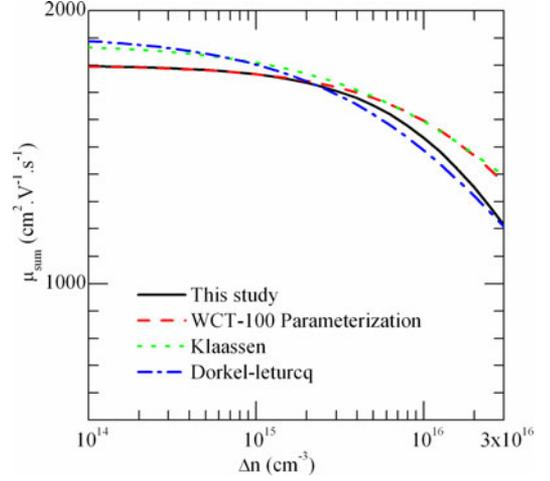
Fig. 6. Comparison of the empirical mobility sum from this study with the existing mobility models from WCT-100 parameterization, Klaassen and Dorkel-Leturcq as a function of injection at 300 K at a doping density of  $4 \times 10^{13} \text{ cm}^{-3}$ .
