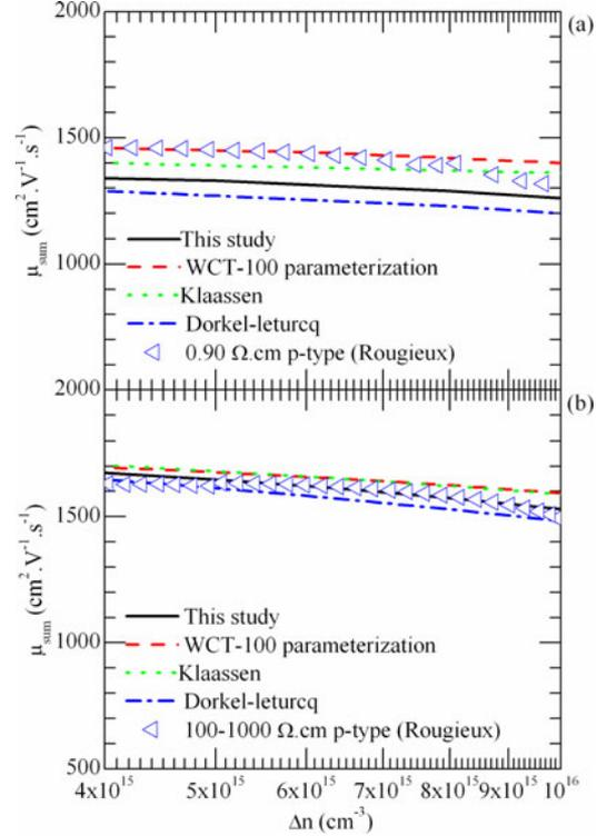
Fig. 9. Comparison of the empirical mobility sum from this study with the existing mobility models from WCT-100 parameterization, Klaassen and Dorkel-Leturcq, and data measured by Rougieux as a function of injection at 300 K for 0.9  $\Omega \cdot \text{cm}$  and 100–1000  $\Omega \cdot \text{cm}$  p-type boron doped silicon.
