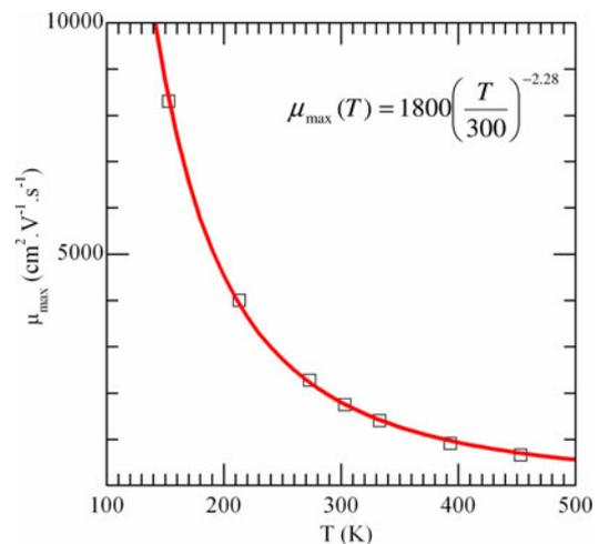
Fig. 4. Temperature dependence of the fitting parameter  $\mu_{\text{max}}$ . This parameter is extracted from the experimental data and subsequently fitted using (4).
