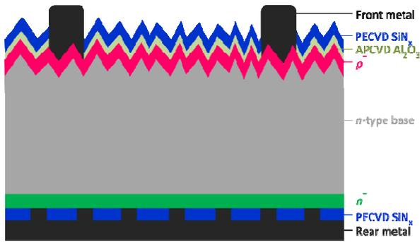
Fig. 1: Schematic cross-section of a high efficiency front-junction  $n$ -type silicon solar cell.
