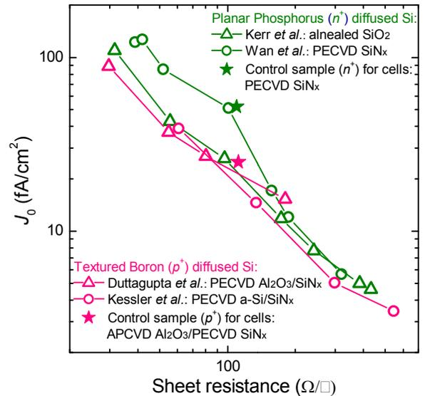
Fig. 2: Effect of sheet resistance on the  $J_0$  of boron ( $p^+$ ) diffused textured surfaces, and on the  $J_0$  of phosphorus ( $n^+$ ) diffused planar surfaces. The results from Duttagupta *et al.* [15], Kessler *et al.* [16], Kerr *et al.* [12] and Wan *et al.* [13] are included for references.
