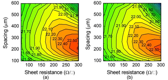
Fig. 4: Contour plot of efficiency as a function of rear dot spacing and rear side sheet resistance for a base resistivity of (a) 3  $\Omega\text{-cm}$ , and (b) 10  $\Omega\text{-cm}$ . The dot size is 40  $\mu\text{m}$ .
