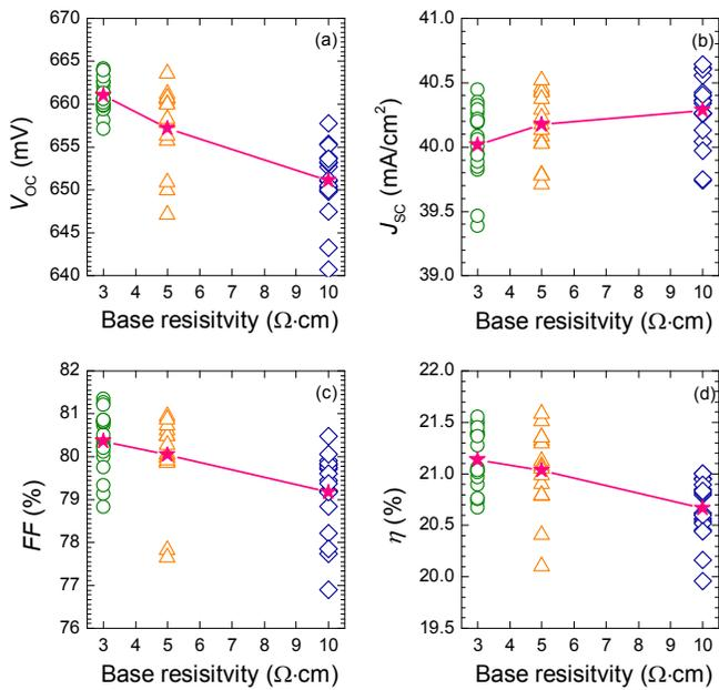
Fig. 3: Effect of base resistivity on small area cell parameters (a)  $V_{OC}$ , (b)  $J_{SC}$ , (c)  $FF$ , and (d) efficiency  $\eta$ . The average is indicated in red stars.
