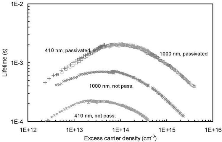
Fig. 6. Effective lifetime as a function of carrier injection level for two high resistivity silicon wafers measured with UV (410 nm) and IR (1000 nm) light. One wafer has passivated surfaces, while the other wafer is not passivated. See details of wafers C and D in Table 2.
