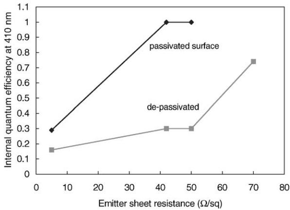
Fig. 5. Internal quantum efficiency at 410 nm obtained from spectral photoconductance measurements for a variety of wafers having different phosphorus diffusions. The 70 Ω/sq diffusion was fabricated in a commercial belt furnace. See Table 2 for details.
