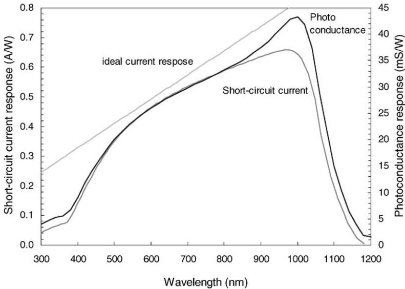
Fig. 2. PC1D simulations for the same case as in Fig. 1, but with a surface recombination velocity of  $S_{\text{front}} = 2 \times 10^5$  cm/s.
