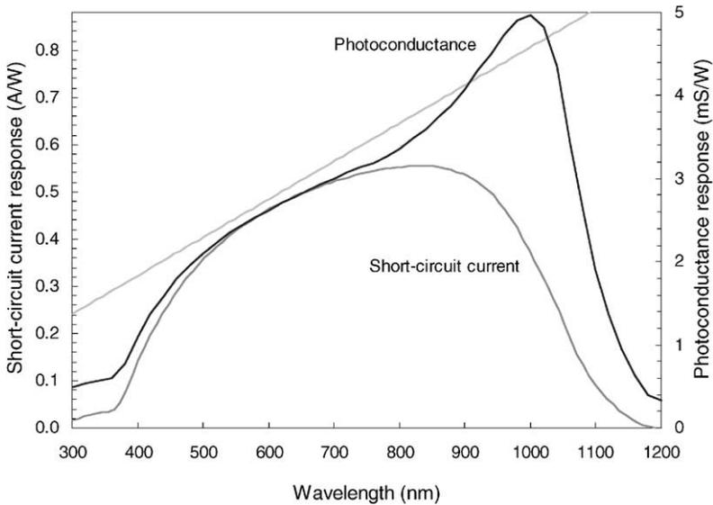
Fig. 3. Spectral photoconductance response and short-circuit current response modelled for the case of a commercial silicon solar cell. Poor current response in the UV and IR are due to emitter and base region losses, respectively. Note that the photoconductance response also shows the UV loss, but not the IR loss.
