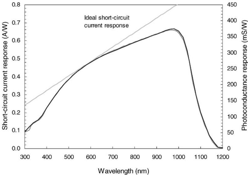
Fig. 1. Modelled spectral photoconductance and short-circuit current as a function of wavelength. The curve shapes are identical for this high-efficiency silicon solar cell structure having a passivated emitter surface ( $S_{\text{front}} = 10^3 \text{ cm/s}$ ). The straight line is the ideal limit of the short-circuit current response.
