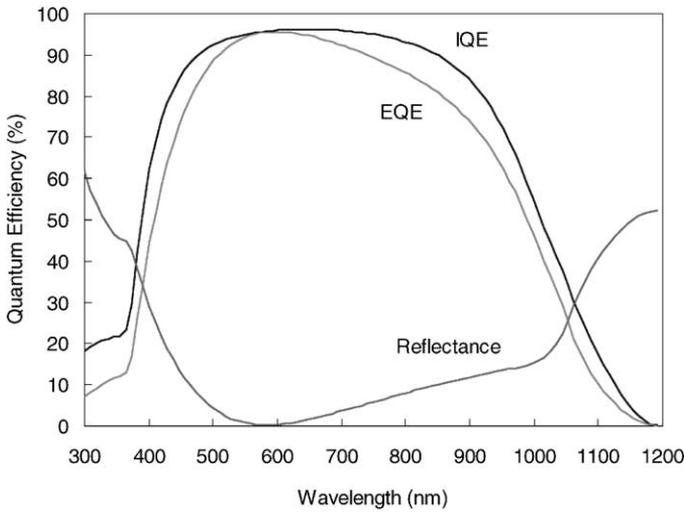
Fig. 4. Internal and external quantum efficiency corresponding to the modelled short-circuit current response of Fig. 3.
