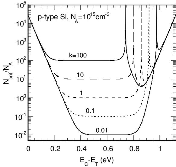
FIG. 3. Values of the low-injection limit of  $N_{crit}$ , normalised with respect to  $N_A=10^{15} \text{ cm}^{-3}$ , as a function of the recombination centre energy level  $E_C-E_T$ . Curves are shown for different values of the capture cross-section ratio  $k$ .
