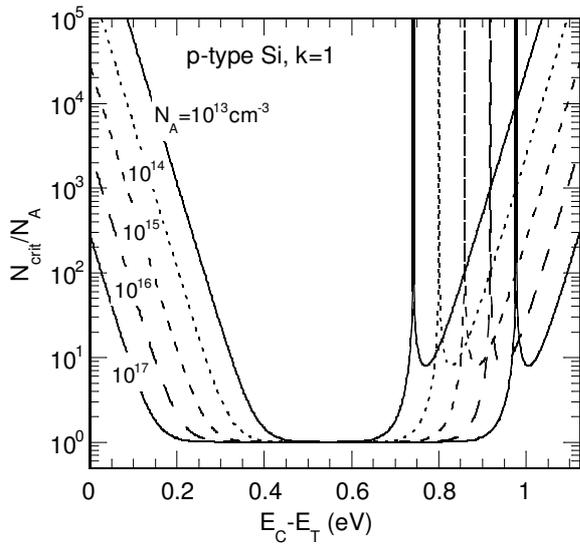
FIG. 4. Values of the low-injection limit of  $N_{crit}$ , normalised with respect to  $N_A$ , as a function of the recombination centre energy level  $E_C-E_T$ . Curves are shown for different values of  $N_A$ . The capture cross-section ratio  $k$  is unity.
