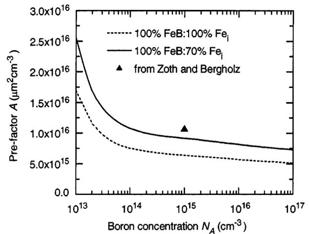
FIG. 3. Comparison of the diffusion length prefactor  $A$  from Zoth and Bergholz with those calculated from the recombination parameters of Table I. The case of 100% FeB before and 100%  $\text{Fe}_i$  after dissociation corresponds to strong optical dissociation, while the 100%:70% case corresponds to the thermal dissociation used by Zoth and Bergholz.
