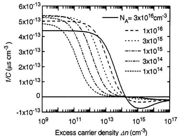
FIG. 1. Inverse lifetime prefactor  $1/C$  versus the excess carrier density  $\Delta n$  for various dopant densities.
