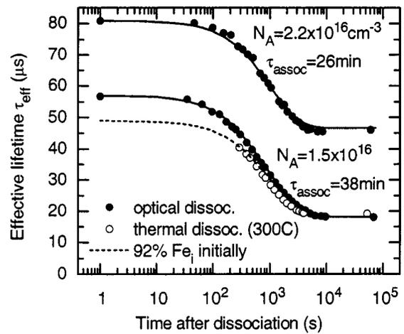
FIG. 5. Decrease of the effective lifetime, measured at  $\Delta n = 3 \times 10^{15} \text{ cm}^{-3}$ , of nongettered mc-Si samples as the FeB pairs re-form after optical or thermal ( $300 \text{ }^\circ\text{C}$  then quenched in water) dissociation. The lines show mono-exponential fits with time constants determined from Eq. (10). For the thermal dissociation case, the proportion as  $\text{Fe}_i$  immediately after quenching is 92%.
