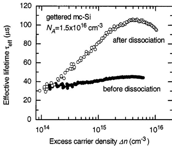
FIG. 4. Effective lifetime versus excess carrier concentration for a partially gettered mc-Si sample containing Fe, showing the crossover of the lifetime curves at  $1.3 \times 10^{14} \text{ cm}^{-3}$  before and after optical dissociation.
