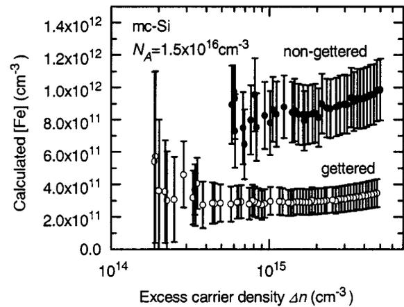
FIG. 7. Calculated Fe concentration  $[\text{Fe}]_{\text{total}}$  for the nongettered and partially gettered neighboring mc-Si samples, revealing that for each sample  $[\text{Fe}]_{\text{total}}$  is independent of  $\Delta n$  within measurement uncertainty.
