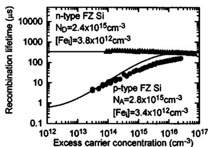
FIG. 1. Modeled and measured lifetimes for  $Fe_i$  in *n*- and *p*-type silicon.
