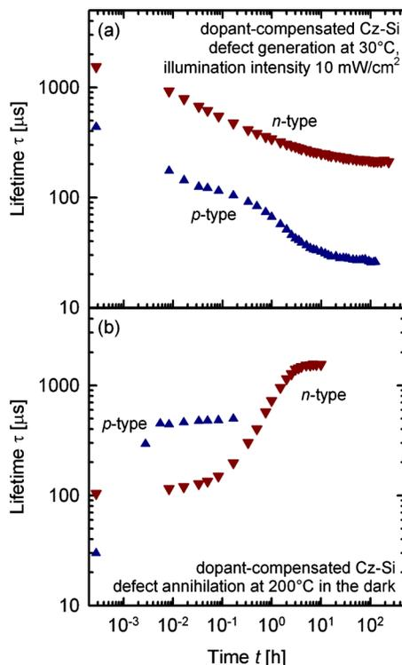
FIG. 1. (Color online) Typical time dependence of the carrier lifetime  $\tau$  in compensated *p*- and *n*-type Cz-Si under (a) 10 mW/cm<sup>2</sup> illumination at 30 °C and (b) at 200 °C in the dark.
