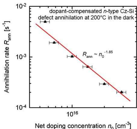
FIG. 7. (Color online) Annihilation rate  $R_{\text{ann}}$  of compensated  $n$ -type Cz-Si samples plotted vs the net doping concentration  $n_0$  on a double-logarithmic scale. The decrease in  $R_{\text{ann}}$  with increasing  $n_0$  can be described by a power law of the form  $R_{\text{ann}} \sim n_0^{-1.85}$ .
