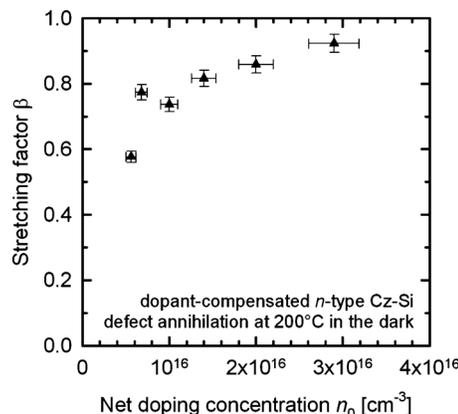
FIG. 8. Stretching factor  $\beta$  obtained from the fits of the defect annihilation rate  $R_{\text{ann}}$  in compensated  $n$ -type Cz-Si (see Fig. 6) plotted vs the net doping concentration  $n_0$ .  $\beta$  increases with increasing  $n_0$ , approaching 1. A stretching factor  $\beta$  of 1 corresponds to a single exponential decay function, which describes the defect annihilation behavior in B-doped  $p$ -type Cz-Si.
