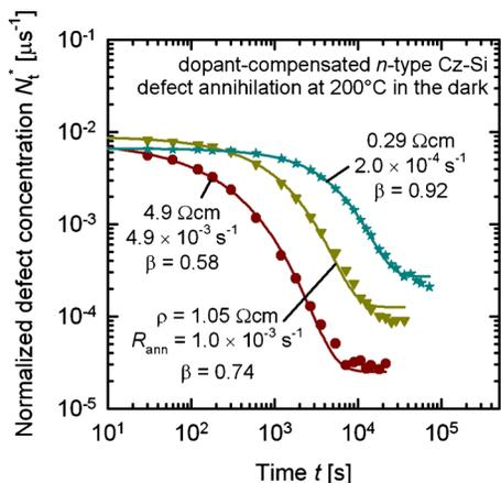
FIG. 6. (Color online) Normalized defect concentration  $N_t^*$  derived from the lifetime data shown in Fig. 5, plotted vs time  $t$  at 200 °C in the dark on a double-logarithmic scale. In order to determine the defect annihilation rate  $R_{\text{ann}}$ , a stretched exponential function of the form  $y = \exp[-(R_{\text{ann}}t)^\beta]$  was fitted to the data.
