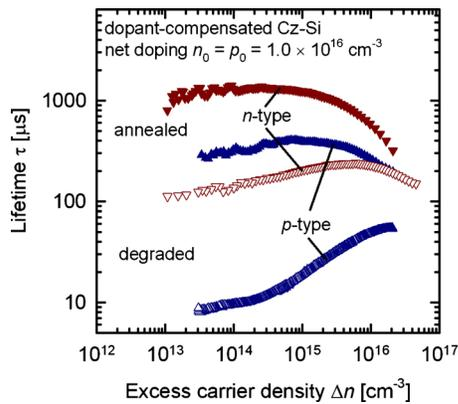
FIG. 10. (Color online) Carrier lifetime  $\tau$  plotted versus excess carrier density  $\Delta n$  in two boron- and phosphorus-doped compensated Cz-Si wafers, one  $p$ -type (triangles up) and one  $n$ -type (triangles down).
