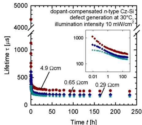
FIG. 4. (Color online) Lifetime  $\tau$  plotted vs duration of illumination  $t$  at 30 °C of three compensated  $n$ -type Cz-Si samples with different resistivities  $\rho$  (and accordingly different net doping concentrations  $n_0$ ). To give a better impression of the early stages of LID, the inset shows the data plotted on a double-logarithmic scale.
