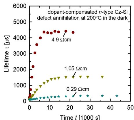
FIG. 5. (Color online) Lifetime  $\tau$  plotted vs time  $t$  at 200 °C in darkness of three compensated  $n$ -type Cz-Si samples with different resistivities. The lifetime after complete defect annihilation increases with increasing resistivity.
