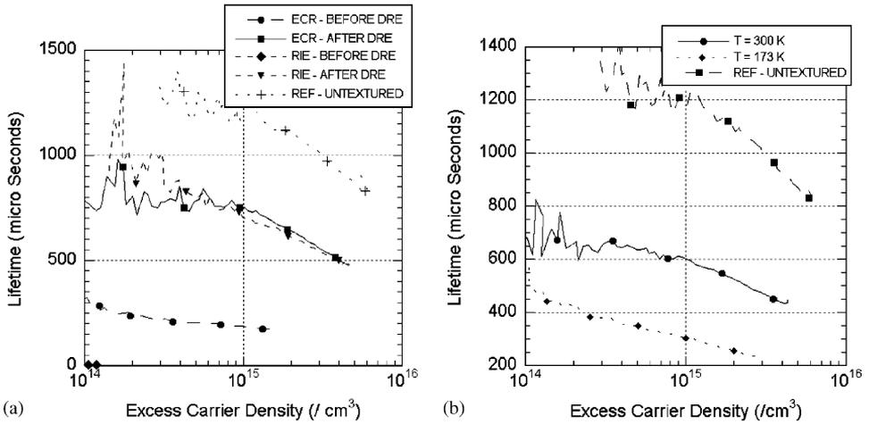
Fig. 3. (a) A comparison of lifetimes of ECR-and RIE-etched Si wafers; (b) Dependence of lifetime on etch temperature.
