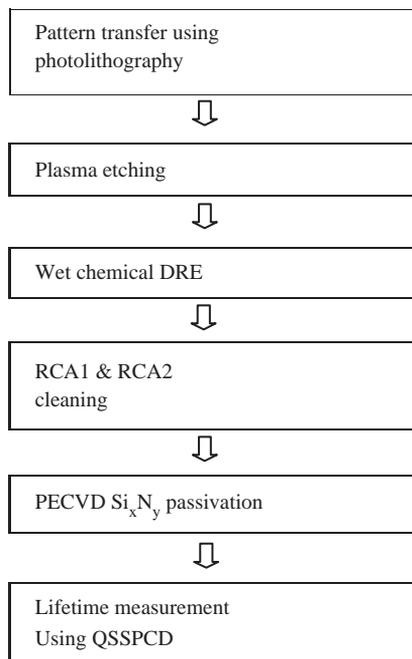
Fig. 1. Schematic of the processes and characterisation involved in plasma-textured silicon wafers.
