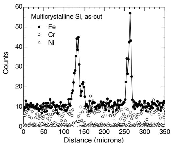
**Figure 2.** Line-scan of the SXRF peak intensities for Fe, Cr and Ni across two Fe-rich particles in an unprocessed multicrystalline silicon wafer.
