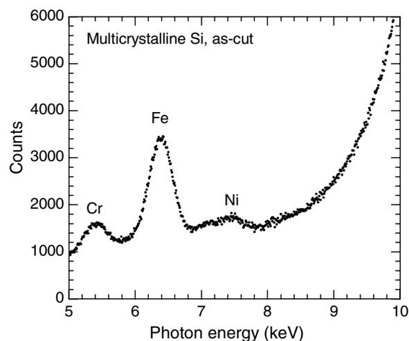
**Figure 1.** X-ray fluorescence spectrum from a region of a multicrystalline silicon wafer containing an Fe-rich particle, with traces of Cr and Ni. The large peak evident at 10 keV is caused by inelastic scattering of the incident beam.
