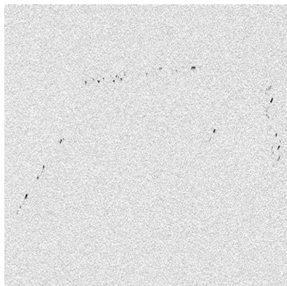
**Figure 3.** The map of Fe particles derived from SXRF spectra in a  $0.72 \times 0.72 \text{ mm}$  region of an unprocessed multicrystalline silicon wafer. The majority of particles are aligned along grain boundaries, as indicated by the linear distributions.
