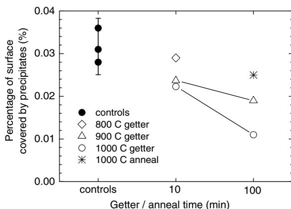
**Figure 5.** Percentage of the surface area covered by detected Fe-rich particles, for unprocessed control samples, and samples that were phosphorus gettered for 10 or 100 min at temperatures of 800, 900 and 1000 °C. The error bars for the control samples represent two standard deviations about the mean. Also shown is a sample annealed without gettering at 1000 °C for 100 min. The lines are guides to the eye.
