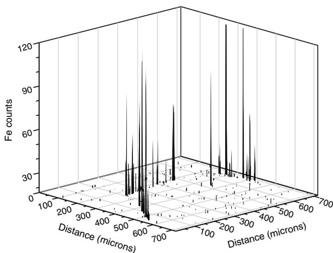
**Figure 4.** Surface plot of Fe SXRF emission intensity for the same region as shown in figure 3. The variations in peak intensity can be caused by different particle sizes and/or depths below the surface.
