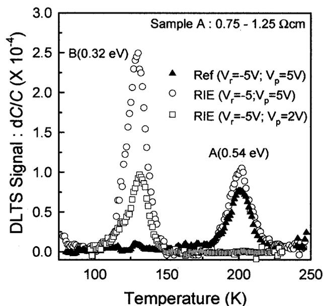
**Figure 3.** DLTS spectra taken from control (solid triangles) and reactive ion etched (open symbols) sample A. The sample had a  $\sim 2 \mu\text{m}$  thick surface layer etched back after RIE. The bias conditions were such that the region extending between  $\sim 0.32$  and  $\sim 0.65 \mu\text{m}$  was probed for the spectrum shown in open squares, whereas the region probed was between  $\sim 0.32$  and  $\sim 0.9 \mu\text{m}$  for the spectrum in open circles.
