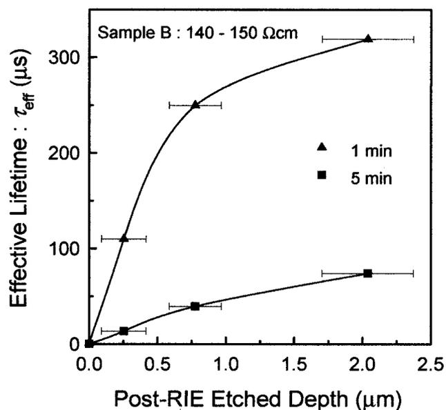
**Figure 2.** Variation of effective lifetime as a function of the amount of Si surface etched back after RIE. RIE was carried out on sample B for either 1 or 5 minutes.
