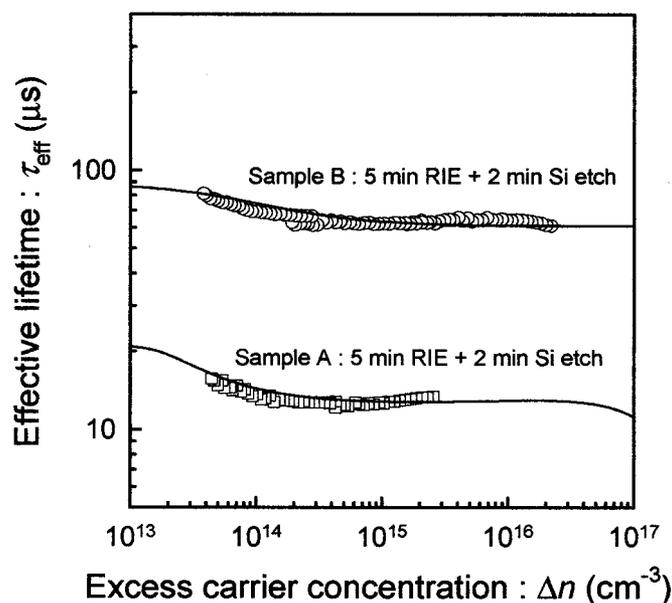
**Figure 5.** Modeling of the injection dependence of the minority carrier lifetimes in plasma-etched samples A and B using the SRH formalism. The solid line for sample A includes the effect of minority carrier trapping centers. The downward curvature of the model at high injection is caused by Auger recombination.
