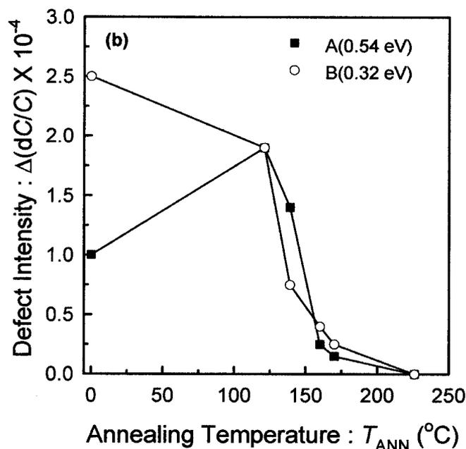
**Figure 4.** (a) Arrhenius plots from which the “signatures” of defects were determined. The data shown in solid symbols show the “signatures” of hole traps previously reported in the literature. (b) isochronal annealing behavior of A (0.54 eV) and B (0.32 eV).
